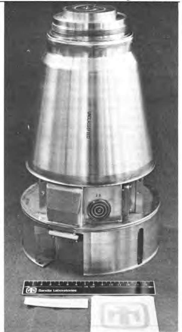
MINIATURIZATION ADVANCES make this complete AF&F (arming, fuzing, and firing) assembly less than six inches across. It is part of the Mk 5 warhead for the Trident II missile.
